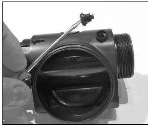
• Use a 3.5 mm screwdriver to remove the plastic locking screw
