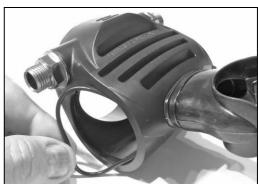
• Fit two new lightly greased O-rings in both ends of the outer body housing
